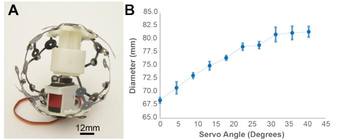
Fig. 3. (A) Internal motor and piston system for the polyhedral auxetic actuator. Since twisting is coupled with extension, inducing an unconstrained twist cause the entire system to expand. (B) We characterize the integrated double-layer actuator by comparing servo angle to actuator diameter.
