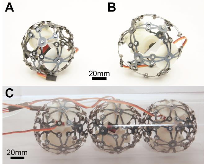
Fig. 1. Overview of electric volumetric actuator in (A) closed state and (B) fully actuated open state. These actuators can be combined modularly in order to build more complex robots, such as (C) a peristaltic tube crawler.
