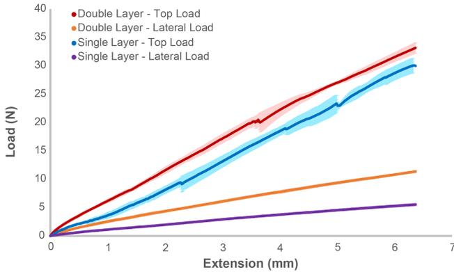
Fig. 4. Compression tests of both single and double layer polyhedral auxetic actuators under top and lateral loading for small deformations in the linear regime. Under both loading conditions, the double layer auxetic performed better than the single layer version, demonstrating nearly twice as much stiffness than the single layer under lateral loading.
