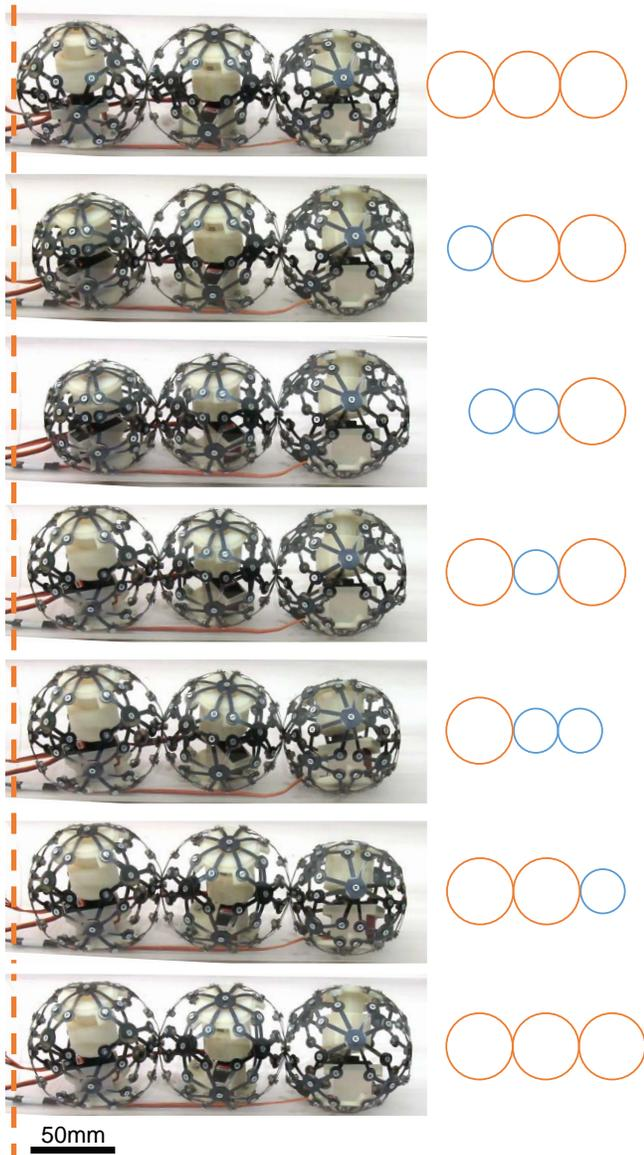
Fig. 5. Three auxetic cells form a tube crawling robot. The sequence pictured here can be used for vertical or horizontal tube crawling. The activated and expanded cells are represented by large orange circles, while the passive collapsed cells are represented by smaller blue circles. The robot depicted here is from a horizontal tube crawl
