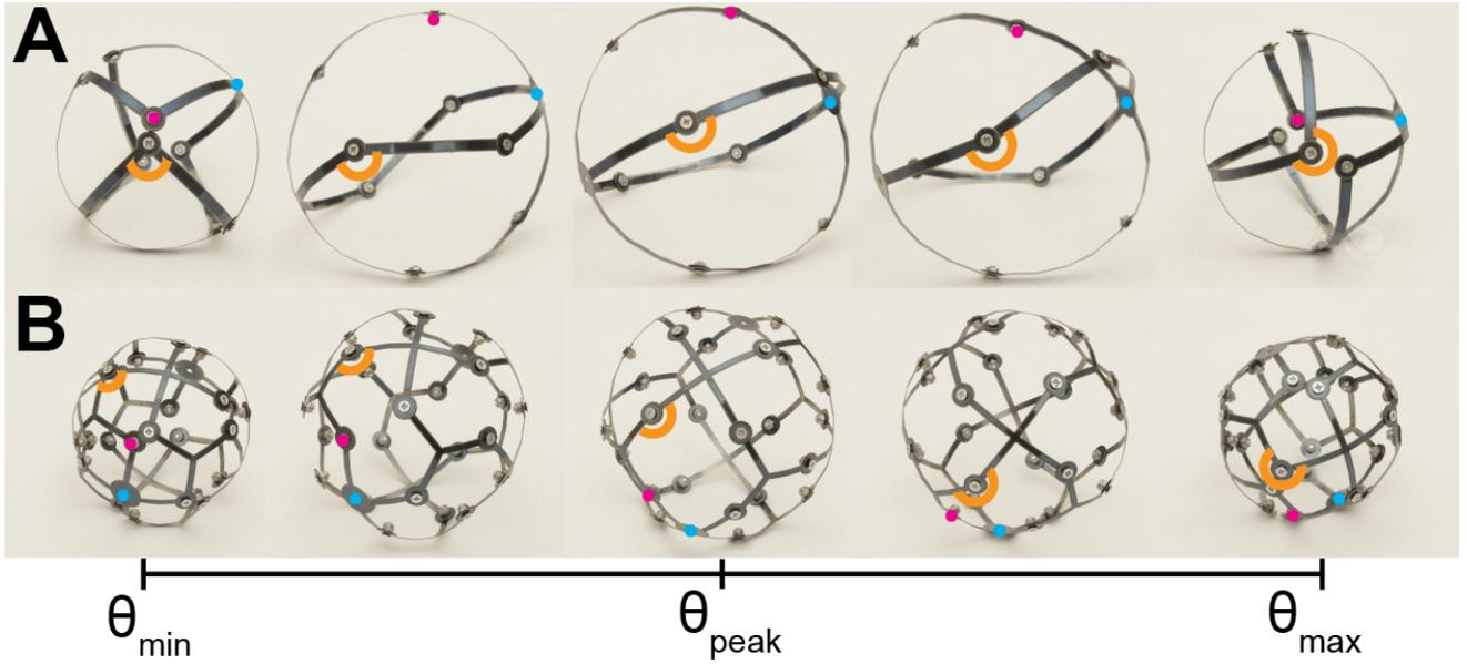
Fig. 2. Open-close trajectories for proposed single-layer skeletons of the point actuators. Both the (A) axial auxetics and the (B) polyhedral auxetics exhibit a twist to open, as can be seen by the change in angle indicated in orange from  $\theta_{min}$  to  $\theta_{max}$ , with maximum open size at  $\theta_{peak}$ . Pink and blue dots have been added to more easily track the movement of the auxetic skeleton.
