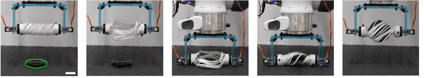
Fig. 7. HSA gripper demonstration, picking up a lens cap (highlighted in green). From left to right, the HSA twists open, the robot lowers onto the object, the HSA is twisted closed, and the robot lift the object up. Scale bar is 2 cm.
